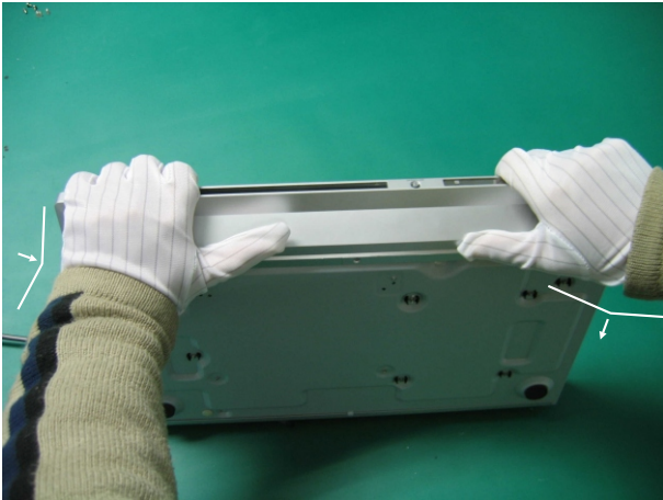
(8) After hearing click sound, press down with wrists forcibly. If you hear a click sound, foot and bottom casing slot are locked. Check whether components reach the proper position.
