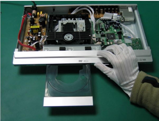
(1) Connect to power supply, switch on power, press OPEN button and disc tray eject.
