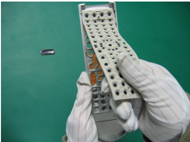
(1) Take hold of remote controller panel by left and , hold electricity conduct glue by right hand and then install it to make sure it reaches the proper position.
