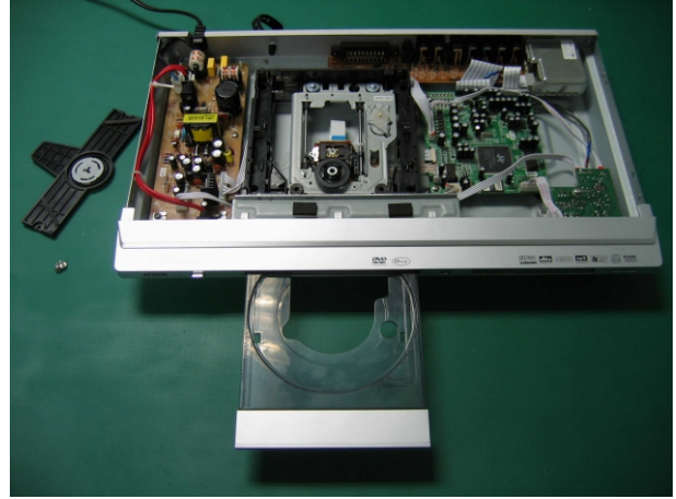
(4) Take out cover board of loader.
