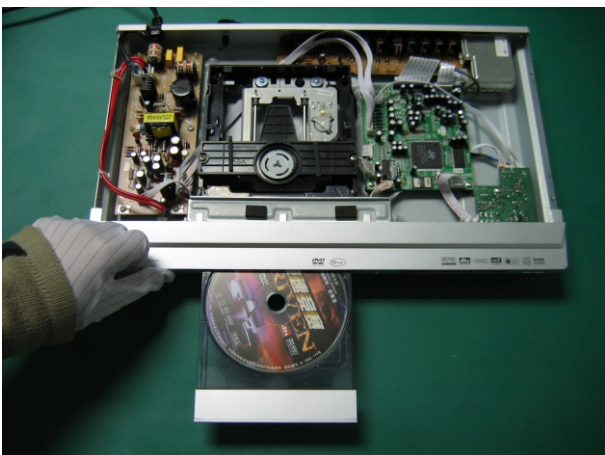
(11) Switch on power, load disc and test functions of the unit.
