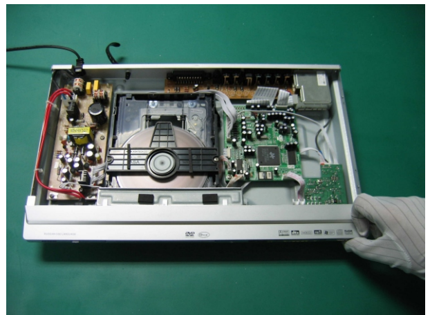
(4) Connect to power supply, switch on power, test functions of the unit and all are ok.
