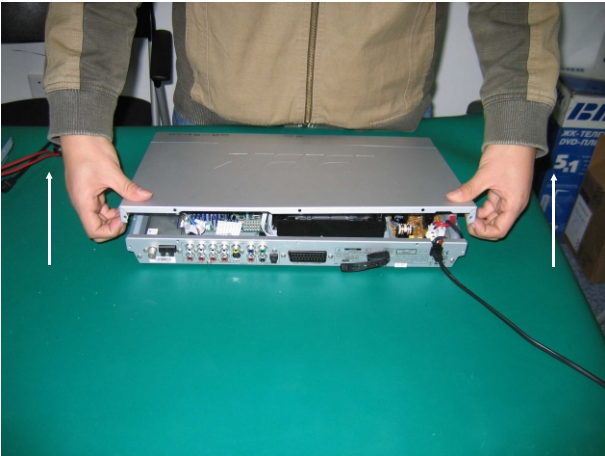
(5) Exert strength continuously by two hands towards the arrow direction (upwards) to lift up the upper cover.
