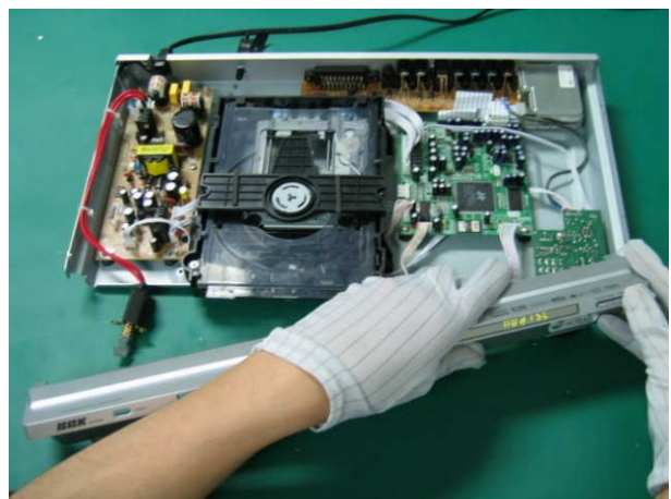
(8) Connect with power supply and switch on power. Hold PC board with four fingers of left hand, and use right hand to test whether function button is sensitive. Switch off power and unplug power cord.
