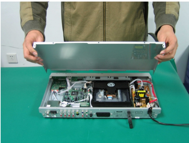
(7) After hearing a click sound, take out the upper cover.
