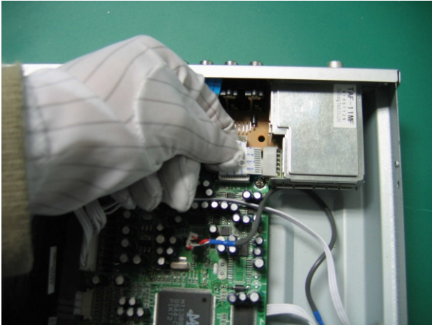
(3) Insert flat cable of AV board components and that of tuner.
