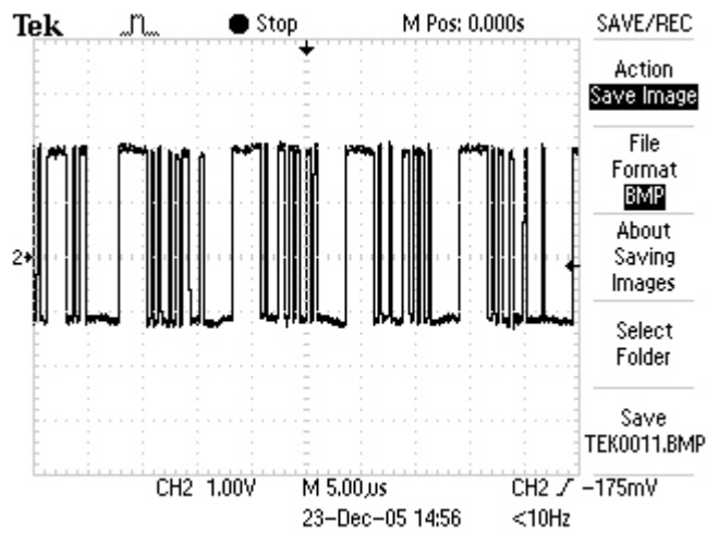
(13) AMDAT: waveform diagram for microphone signal after 5340 A/D conversion
