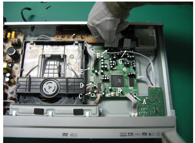
(2) Insert flat cable A, B, C, E, F, G.
