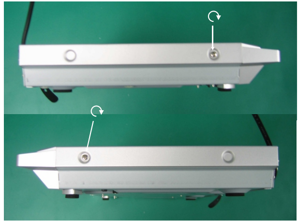
(6) Use electric screwdriver or "+"-shaped screwdriver to fix screw on left and right hand side of the upper cover.
