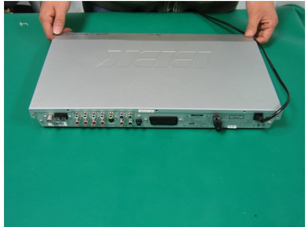
(4) After well installing the upper cover, check whether the whole upper cover has reached proper position.
