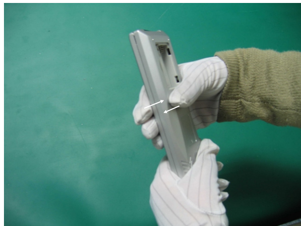
(6) Afteraiming at bottom position of remote controller, left hand to hold the bottom partforcibly. Hold the middle part of remotecontroller with thumb and another four fingers of right hand and press towards the same direction forcibly untilyou hear a click sound.
