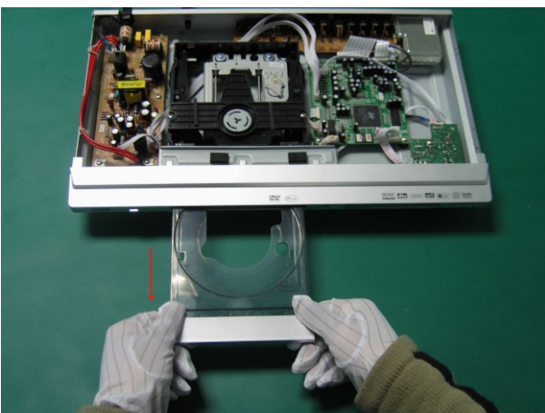
(3) After hearing a click sound, exert strength towards arrow direction (outwards) by two hands and the door falls off naturally.
