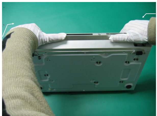
(8) Take hold of control panel components and press down with wrist forcibly towards the arrow direction. After hearing a click sound, the panel and bottom casing slot are locked.
