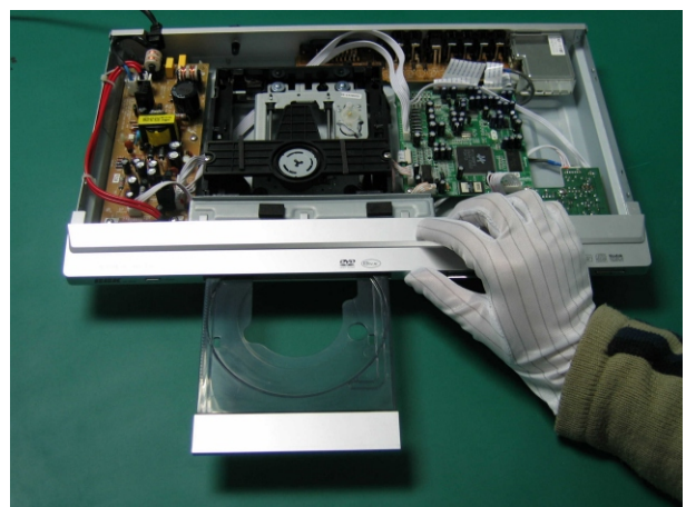
(2) Turn on power, press OPEN/CLOSE button and disc tray ejects. Turn off power and unplug power cord.
