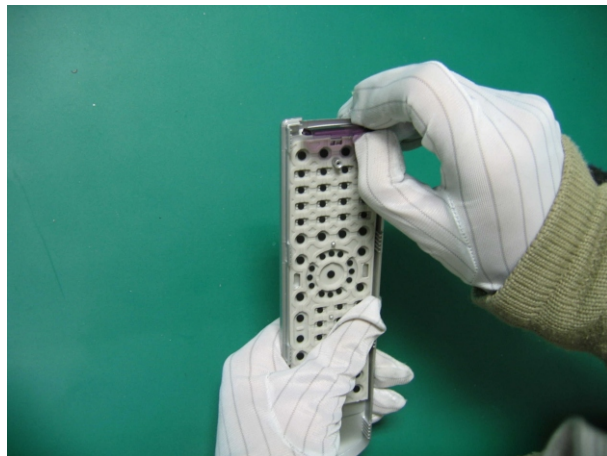
(2) Take hold of remote controller frontpanel by left hand, take glass between thumb and forefinger of right hand and insert into slot.
