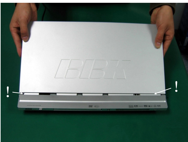
(1) Take hold of the upper cover by two hands at an angle more than 45-degree, then take the front edge of the upper cover aiming at the slot and push it slightly to the position.
