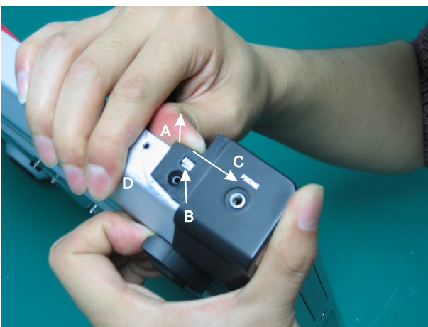
(5) Take hold of panel by left hand, and press bottom casing D by four fingers of right hand. Use thumb to hold panel button bracket and exert strength towards direction of arrow A (outwards) until panel falls off from bottom casing button B, then exert strength towards direction of arrow C, and panel on left hand side falls off from bottom casing.
