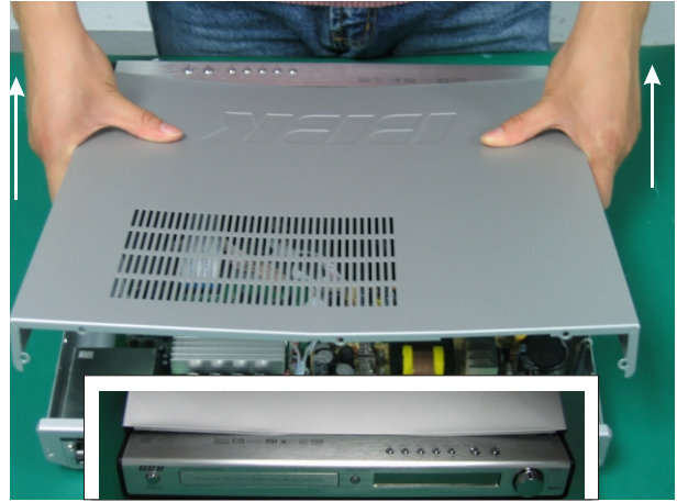
(6) After uplifting upper cover, move two hands to the middle part of upper cover and hold it with thumb unchanged and exert strength towards arrow direction by the other four fingers until the front edge of two sides of upper cover falls off from the joint of panel.
