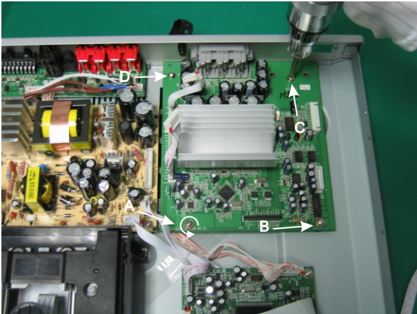
(7) Use electric screwdriver or "+"-shaped screwdriver to unfix screws A, B and C of power amplifier board.
