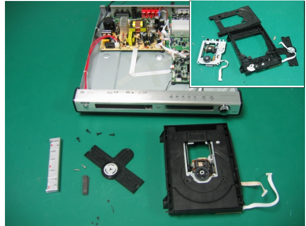
(10) Take out loader components. If you still want to separate loader with frame, please refer to section 4.2 -- Loader, shown as small figure.
