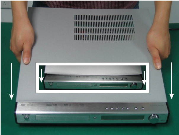
(3) After the middle part of front edge of upper cover reaches the proper position, exert strength to press down towards arrow direction (downwards) by two hands until the two sides of front edge of upper cover fasten the button of panel.
