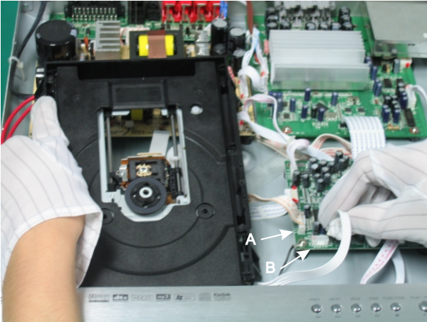
(9) Take hold of loader components by left hand and unplug flat cable A, B by right hand.
