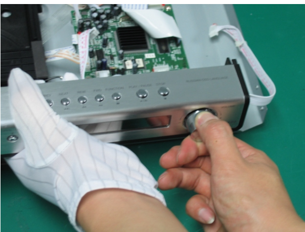
(3) Take hold of panel by left hand and press PC board with the left four fingers. Take the outside decoration knob of "volume" knob between thumb and forefinger of right hand, and then exert strength to push in to reach proper position. The rotation should not have obstruction.
