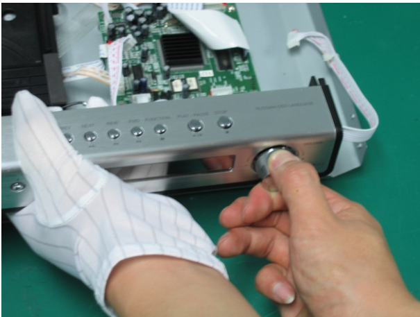
(9) Take hold panel by left hand, take volume button between thumb and forefinger of right hand and pull out outside decoration knob.
