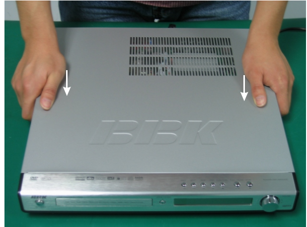
(4) After the front edge of upper cover fastens fully, put down upper cover by two hands until the back edge of upper cover joints with bottom casing automatically. Check whether the entire upper cover has reached the proper position.
