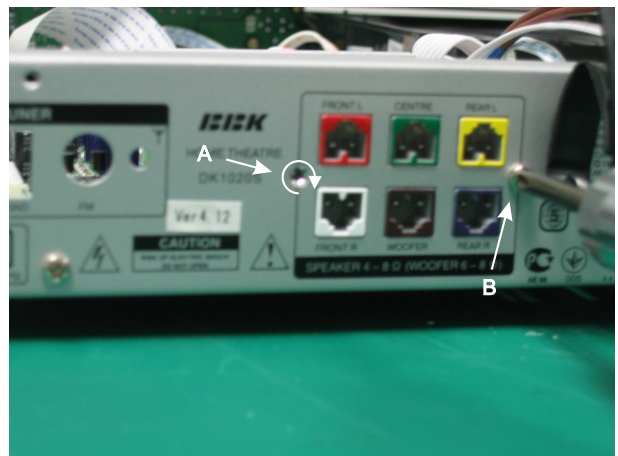
(2) Use electric screwdriver or "+"-shaped screwdriver to fix screws A and B of rear cover of power amplifier board.
