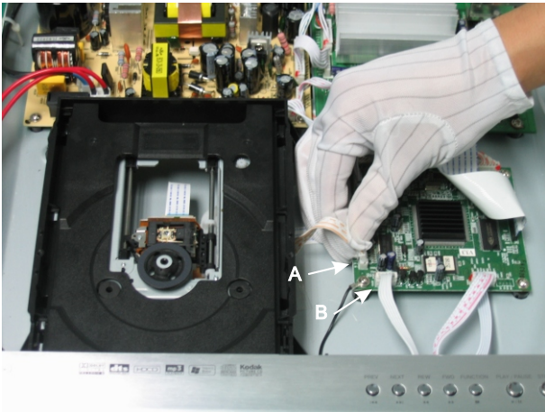
(5) Insert loader components flat cable A and B.
