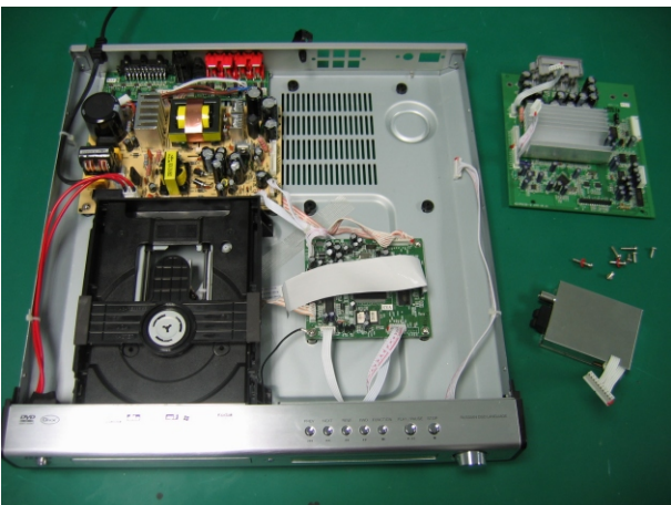
(1) Before assembling power amplifier board, place the power amplifier board to proper position.
