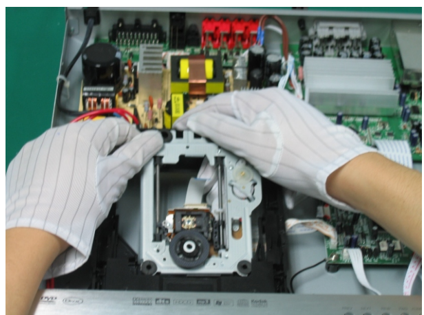
(4) Take flat cable between forefinger and middle finger of right hand, then thumb and forefinger of left hand take the flat cable and place loader to proper position by right hand.
