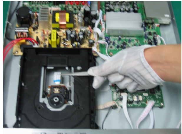
(2) Take hold of forceps by right hand and then wiggle out laser head flat cable.
