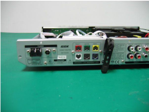
(1) Before disassembling power amplifier board, disassemble tuner firstly.
