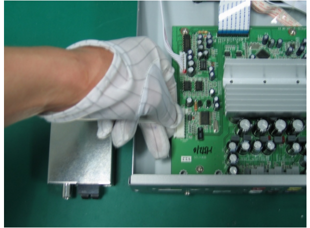
(6) Insert flat cable of tuner.
