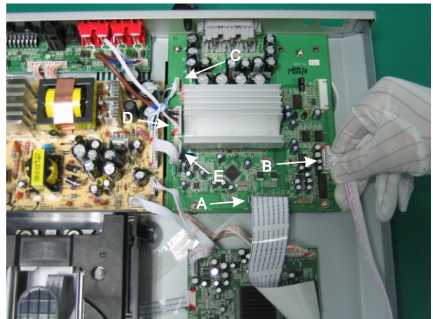
(4) Insert flat cable A, B, C and D on power amplifier board.
