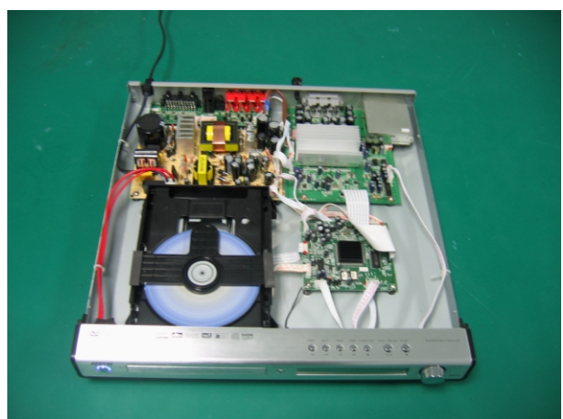
(10) Connect to power supply, switch on power and test functions, which are all normal.
