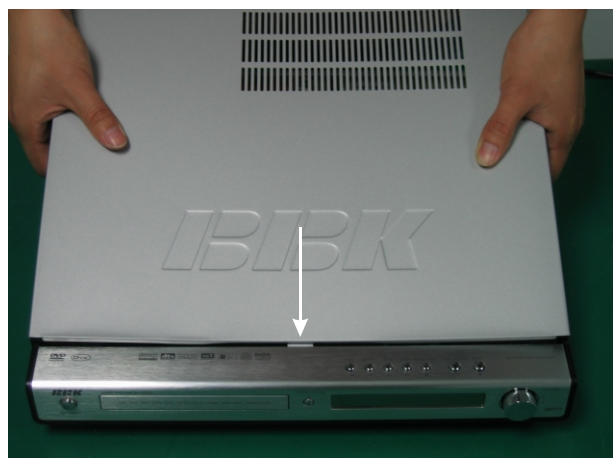
(2) After taking hold of the upper cover with its concave, aiming at the slot, push the middle part of the front edge of upper cover slightly at an angle of mote than 45-degree to its proper position.
