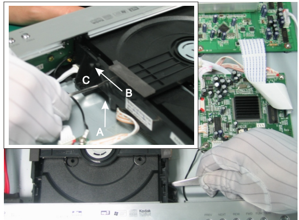
(2) Take hold of tweezers by right hand and insert into the bottom part of loader components. After holding towards arrow direction (upwards) to top part, keep the height and then slide towards direction of arrow B until point C.
