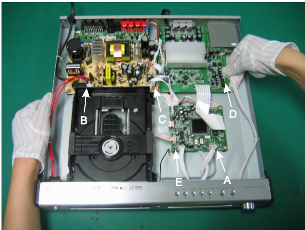
(7) Insert flat cable A, B, C and D. Use electric screwdriver or "+"-shaped screwdriver to fix panel grounding wire E.
