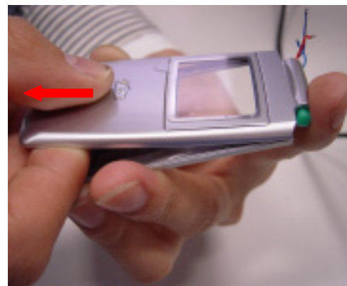
7. Use a plastic screwdriver to slide and open the gap between the folders. Then detach them carefully with both hands.
