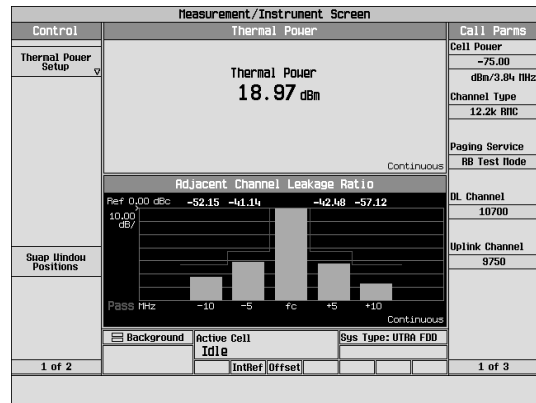
Fig. 4-20-8 Output Level at Isolator Output (N303.Out)
