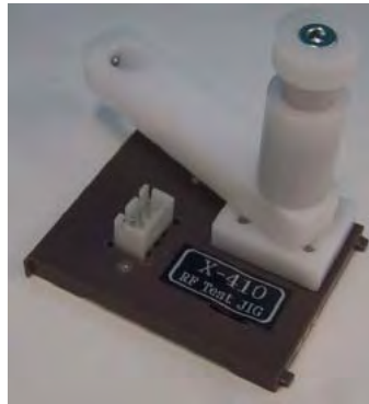
Figure 5.2. : Dummy Battery with RF Test Jig
