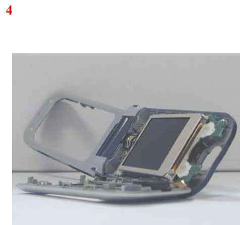
Set a protection film on the main LED to avoid dust contamination and fingerprints
