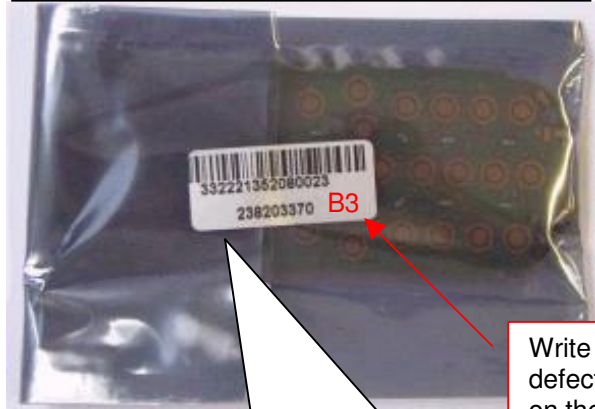
ESD shielding bag closed by the IMEI label
