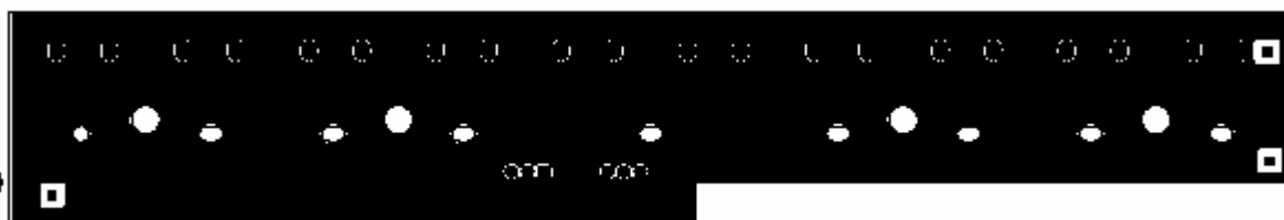
Keypad board 3479C(Top layer view)
